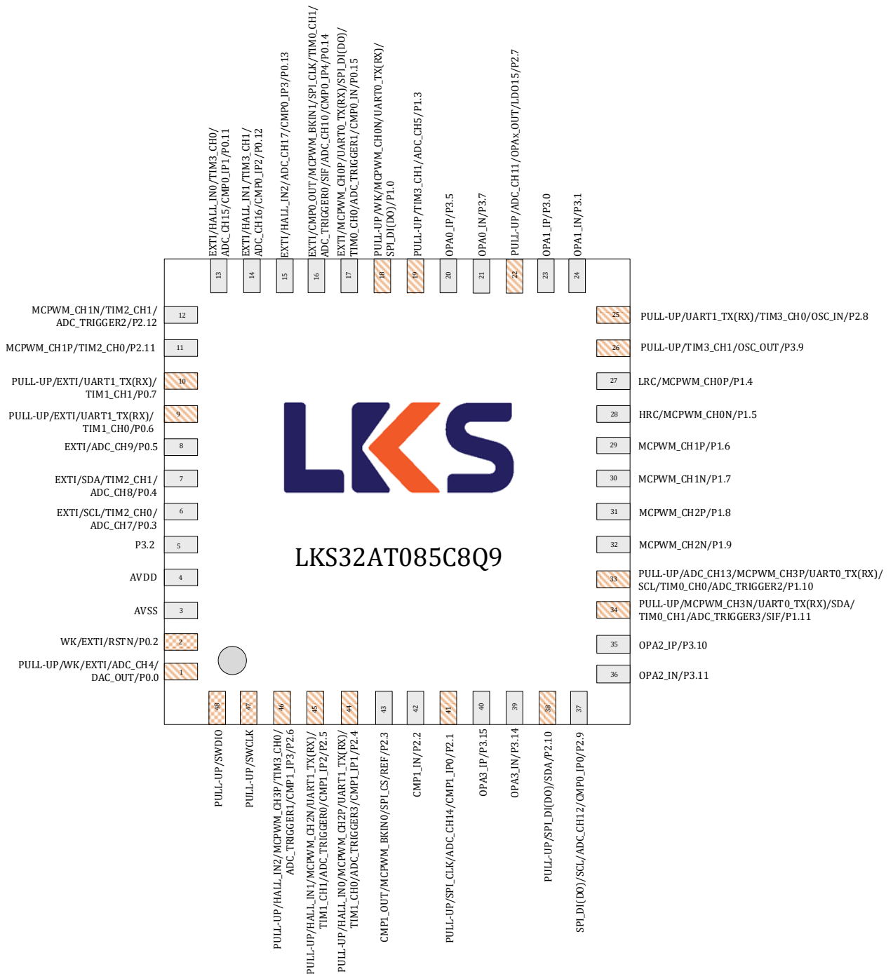
Fig. 3-5 LKS32AT085C8Q9 Pin Assignment
