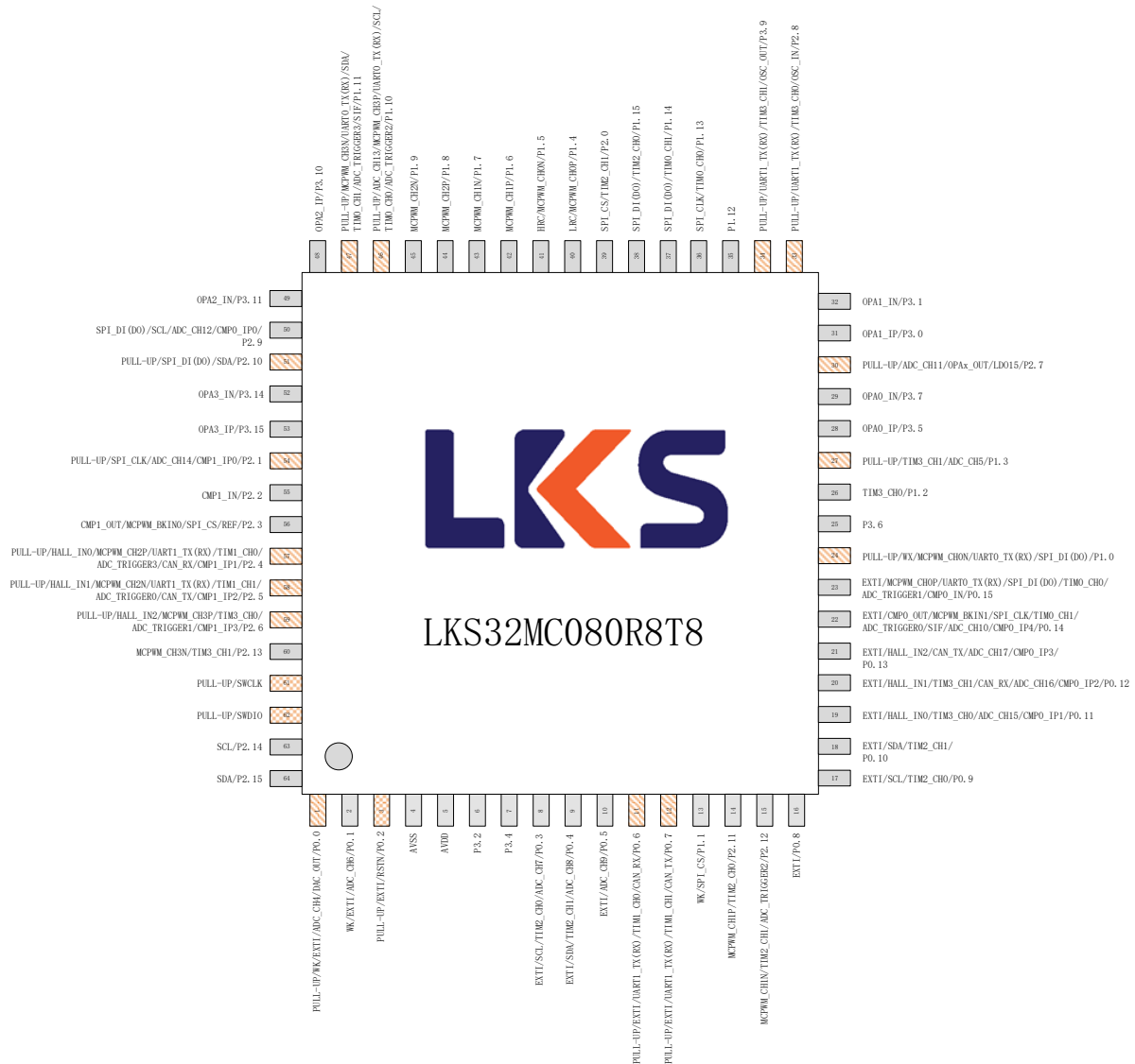
Fig. 3-1 LKS32MC080R8T8 Pin Assignment
